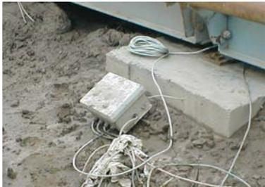
Eliminating junction boxes eliminates a common cause of scale failure.
